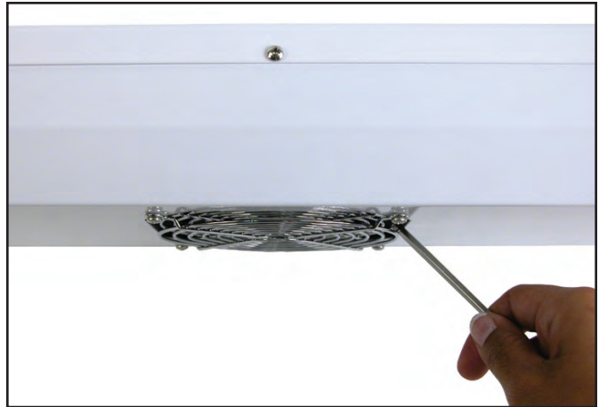
Figure 8. Shorting the ionizer's two fan grills
